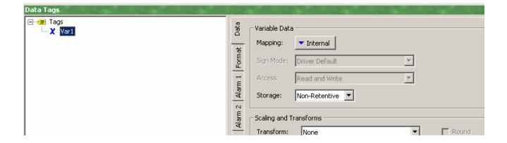
7) Select the "mapping" and then select the device you want to connect to which in this case is DRV1.
